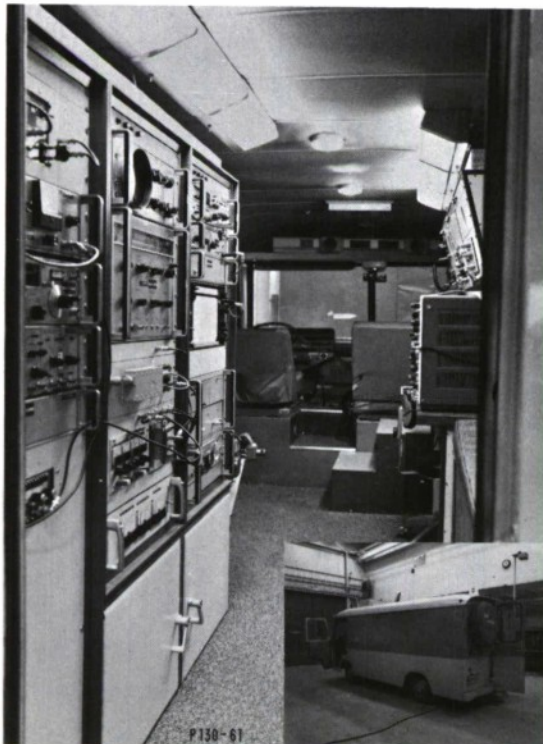
Fig. 2. Mobile test facility for measurement of transponder interference.
